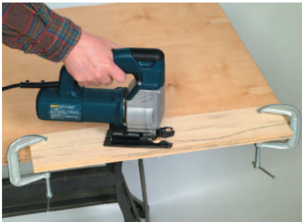
Figure 5-27 Cutting a Curve
