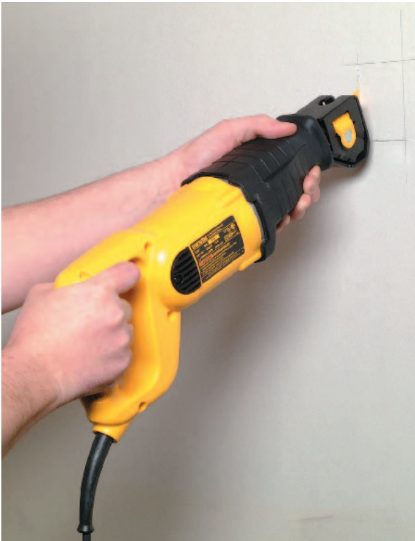
Figure 5-30 A Reciprocating Saw Hand Position The saw should be controlled with two hands. Hold the shoe (the baseplate) firmly against the material being cut.
