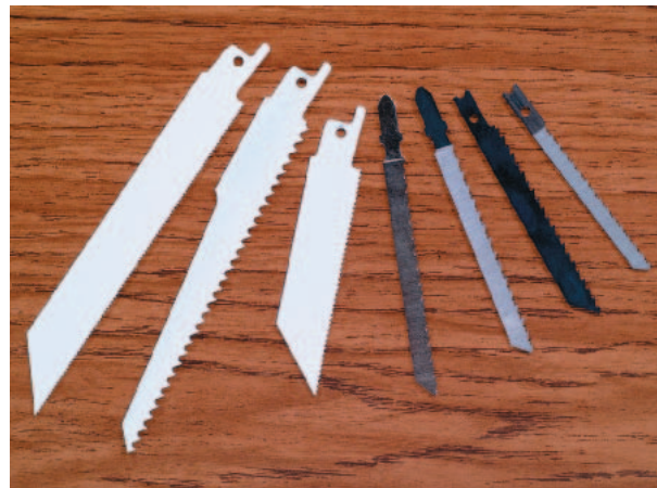
Figure 5-31 Straight Blades Various Sizes The wide blades are for reciprocating saws. The narrow blades are for jigsaws.
