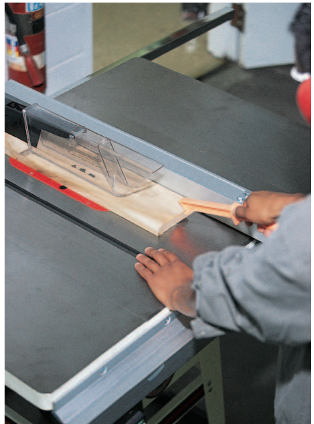
Figure 5-15 Ripping Narrow Stock Use a Push Stick Note that the push stick is used between the blade and the fence, not on the outside of the blade. The guard should be in place for all tool operations.
