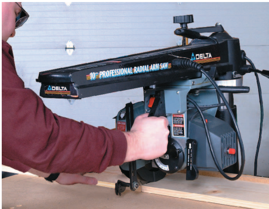
Figure 5-24 Hand Position Keep the Saw from Lurching The proper hand position for crosscutting. Notice the position of the anti-kickback fingers. The guard should be in place for all tool operations.
